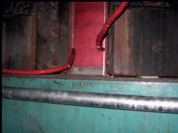
Electrical connections of the SAVESEARCH<sup>®</sup> electrodes on a 10 t furnace
