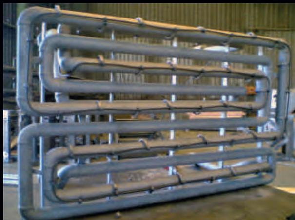
Sensor installation on the cooling water system of a copper block before casting
