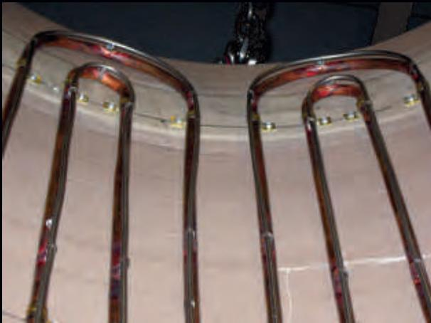
Heat shield of graphitisation furnace, sensor type 1
