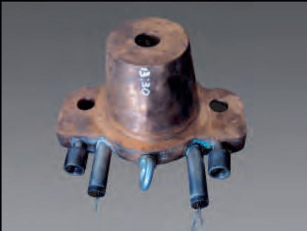
Water cooled copper module of a slag tap hole with integrated OPTISAVE sensors
