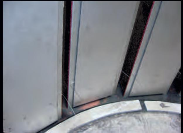
Detail of SAVESEARCH<sup>®</sup> electrodes in a vacuum furnace
